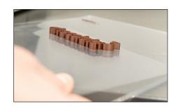
Note: We recommend not to remove the print objects on the print bed (2), but to remove the build-plate (3) and remove the objects on a solid surface.
