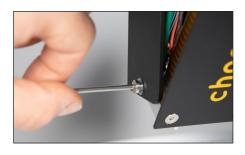
Loosen the screw (19) and push the tube (17) up a little.
