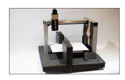
Remove the front and rear foam by pulling on it while holding the print bed (2).
