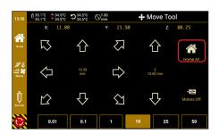
All motors can be switched off via the button. The individual axes can now be moved carefully by hand.
