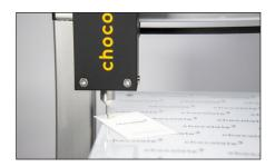
If necessary, adjust the distance with the knurled screw on the left. This causes the entire print bed to tilt to the left or right. Repeat the process until the distance is the same along the entire width of the print bed.
