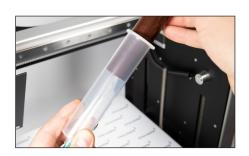
Insert the prepared cartridge into the print head (1).
