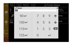
Under Flow, the material feed can be set as a percentage. 100% corresponds to the material feed set in the .gcode.
