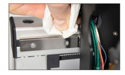
Clean the linear guides from dirt and excess grease.
