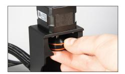
Make sure to screw the piston on completely, otherwise the height of the empty point of the cartridge may not be correct.
