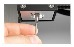
Replace the matching nozzle element (14) from below and tighten the two screws (20).
