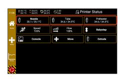
Under Speed, the print speed can be set as a percentage, with 100% being the speed set in .gcode.
