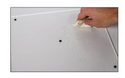
Place a foil in the middle of the buildplate (3) and smooth it out. From the centre, brush out as many air bubbles as possible.
