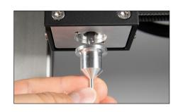
Replace the nozzle by unscrewing and screwing it back on.
