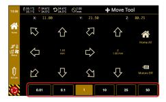
The button can be used to trigger a homing of all\* axes.
