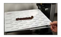
Depending on the ambient temperature, the chocolate needs another 1-10 minutes to finish crystallising. A completely solid chocolate is the basis for removing the print objects. If necessary, briefly place the buildplate (3) in a cool place.
