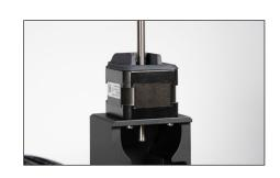
Unscrew the spindle upwards in an anti-clockwise direction.
