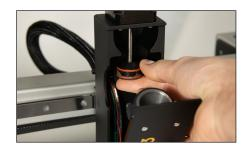
To keep the print head (1) clean, it may help to wrap a piece of paper around the piston (15) while removing it.
