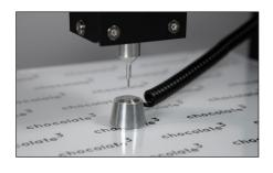
Confirm that the Z button (6) is under the nozzle.
