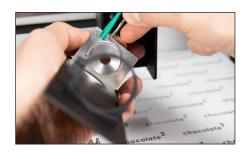
Make sure that the cables of the tube (17) point towards the remaining cables in the left rear corner.
