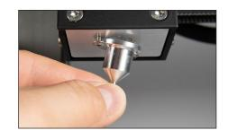
Replace the nozzle on the cartridge by unscrewing and screwing it back on.
