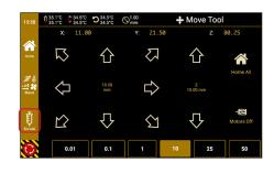
In the lower part, the distance to be travelled can be selected per tap.
