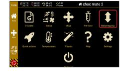
Opens the page for correcting the nozzle buildplate distance. See also chapter 5.9.3.
